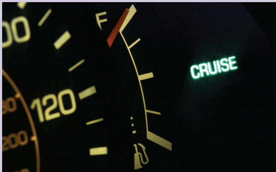
Figure 1.1 Hypermiling dramatically reduces gas consumption in a car. One of the ways to implement hypermiling is using a cruise control system to maintain a constant speed.
